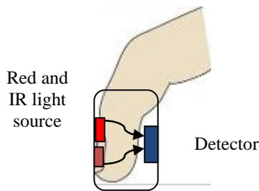
**Fig 1: The red and infrared light being shone through the finger**
