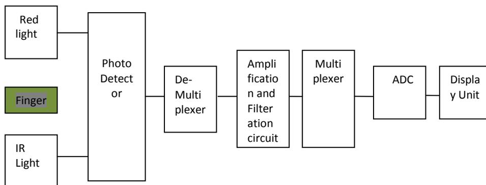
**Fig 2: A schematic diagram of a OGH monitor**
